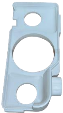
DEVELOPMENT OF GABLE (INVESTMENT CASTING) BY 3D PRINTING Gun Carriage Factory, Jabalpur
