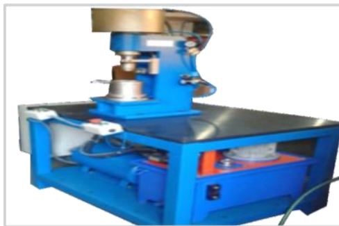
CAULKING EQUIPMENT Machine tool prototype factory, Ambernath
